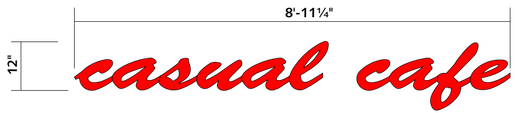
B CHANNEL LETTER LAYOUT (FLAT VIEW)
